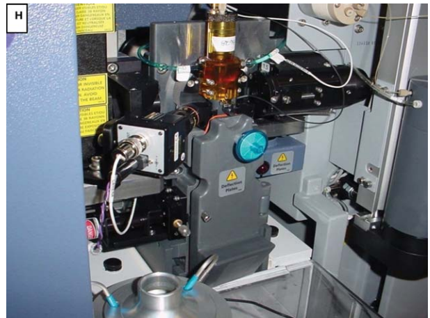
Figure H. Impactor placement. On top of collection chamber, door partially open.
