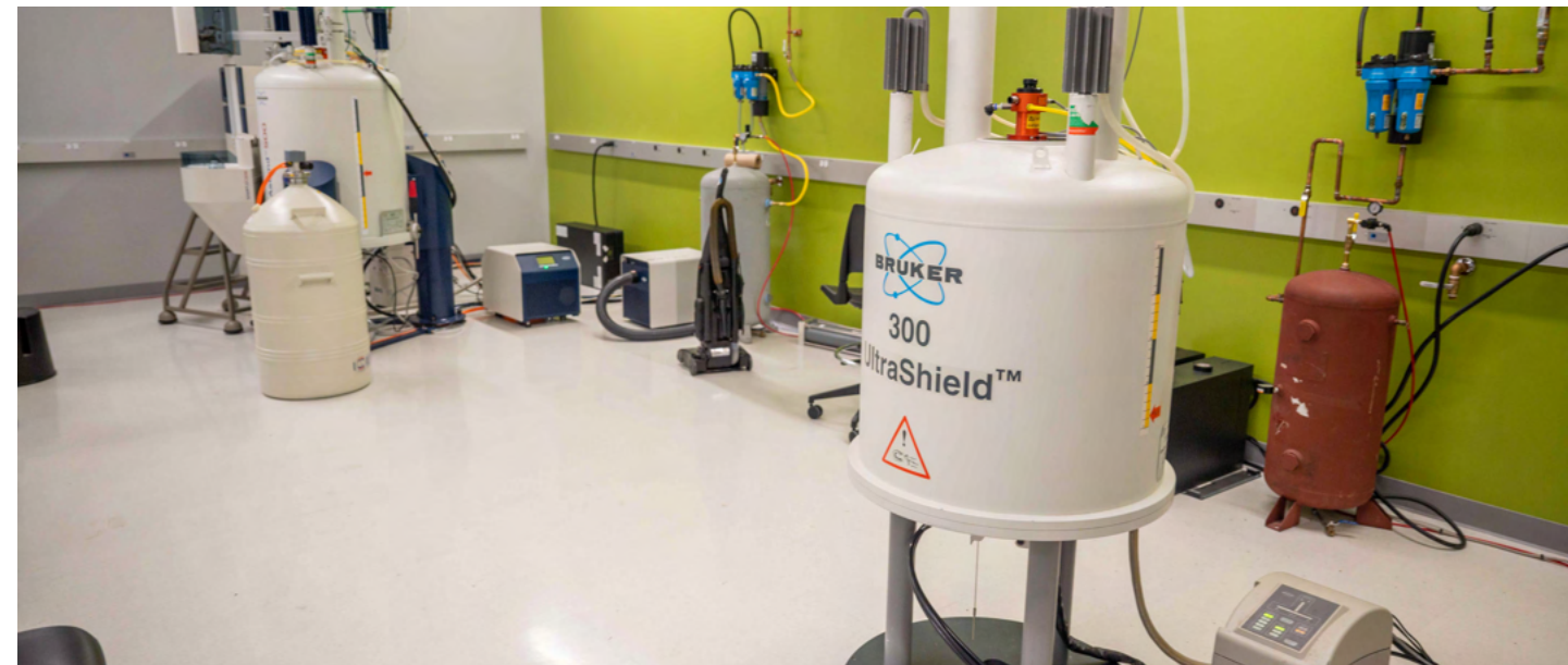
Nuclear Magnetic Resonance (NMR) instruments set up on the fourth floor (above).
